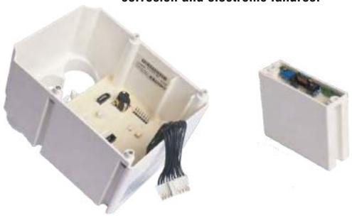
Major failures are seen in electronics mainly due to moist instrument air or external humidity, damaging the exposed electronic parts.
