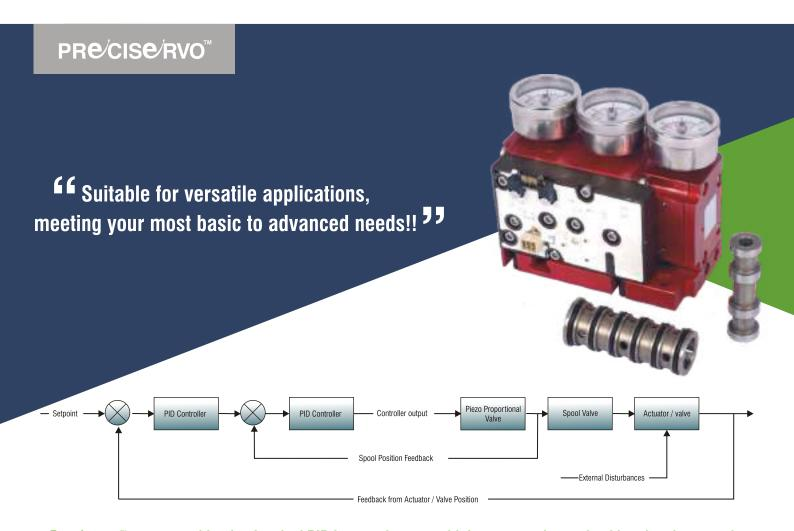
Pre cise rvo™ operates with adaptive dual PID loop and ensures high accuracy, lower dead band and extremely steady performance of positioner. Primary loop is controlling the spool position of Pre cise rvo™ and secondary loop is controlling the actual position.
